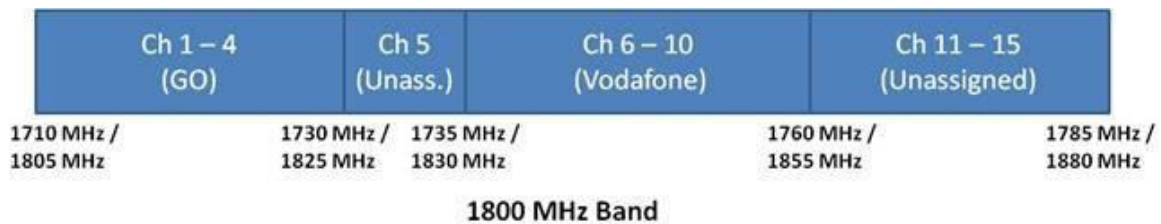
FIGURE 1: CURRENT SPECTRUM ASSIGNMENTS IN THE 1800 MHz BANDS
